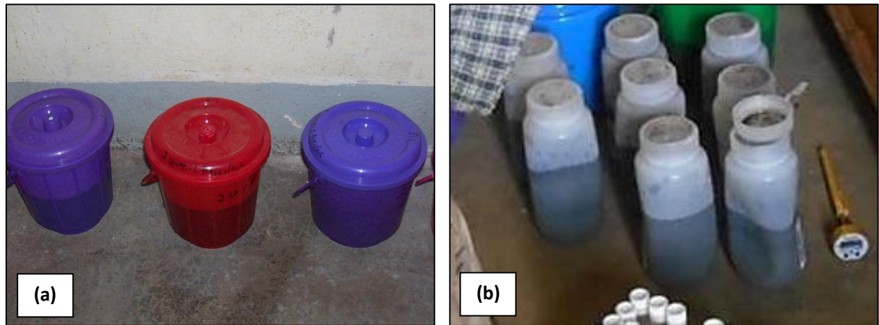
Figure 8: Containers used during ammonia treatment tests. (a) Two-liter buckets used during stage 1 (photograph taken by the author); (b) 500-milliliter bottles used during stage 2 (photograph taken by Debra Trimmer).
